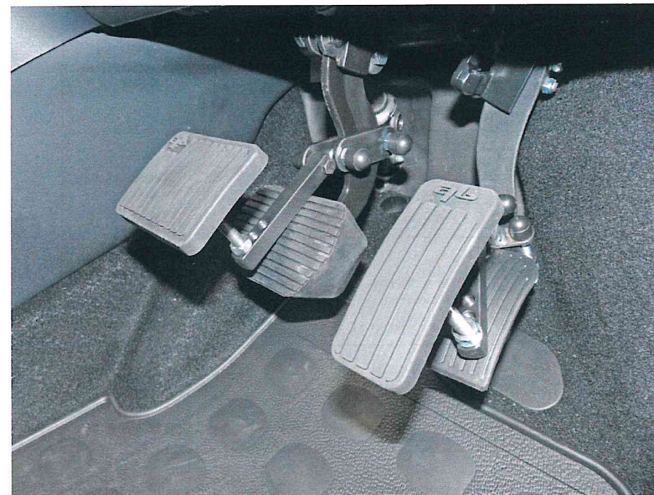
Brake & Accelerator Pedal Extension fitted to 2012 model Citroen DS3
